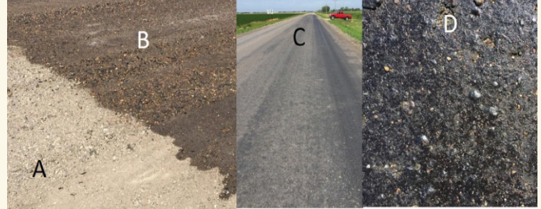
A) Untreated gravel. B) 30 minutes after treatment. C) After 6 weeks D) Close up of treated road surface. (Actual test conducted on gravel with a 25% asphalt regrind mixture).
